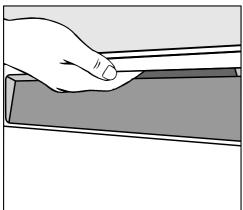
To open the door, reach under the door grip and pull.
