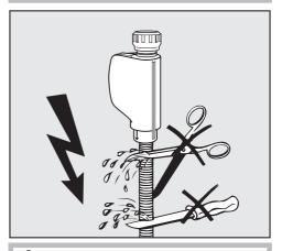
The inlet hose must not be shortened or damaged in any way as it contains electrical components (see illustration).
